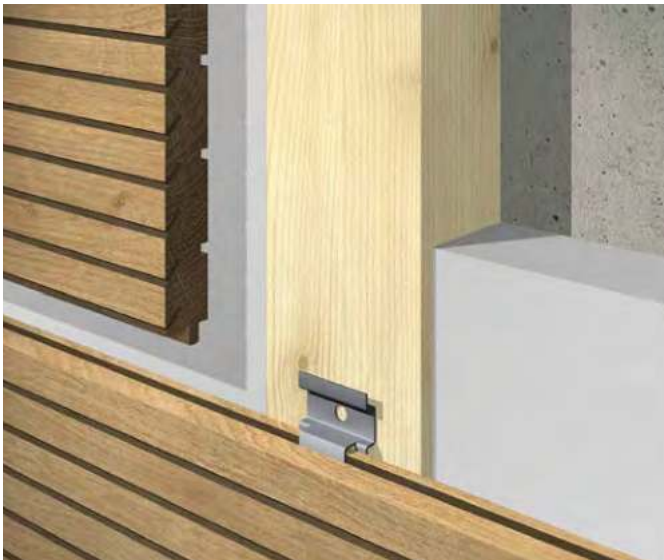
Detail horizontal mounting with mounting clip.
