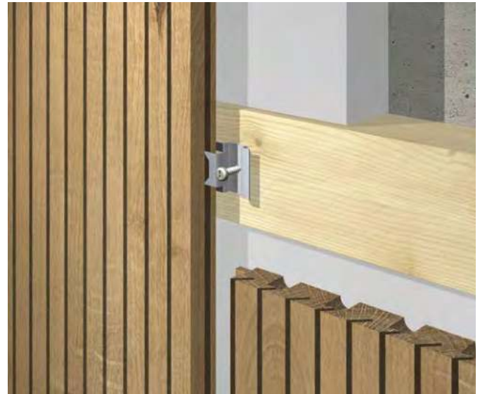
Detail of vertical mounting with mounting clip.
