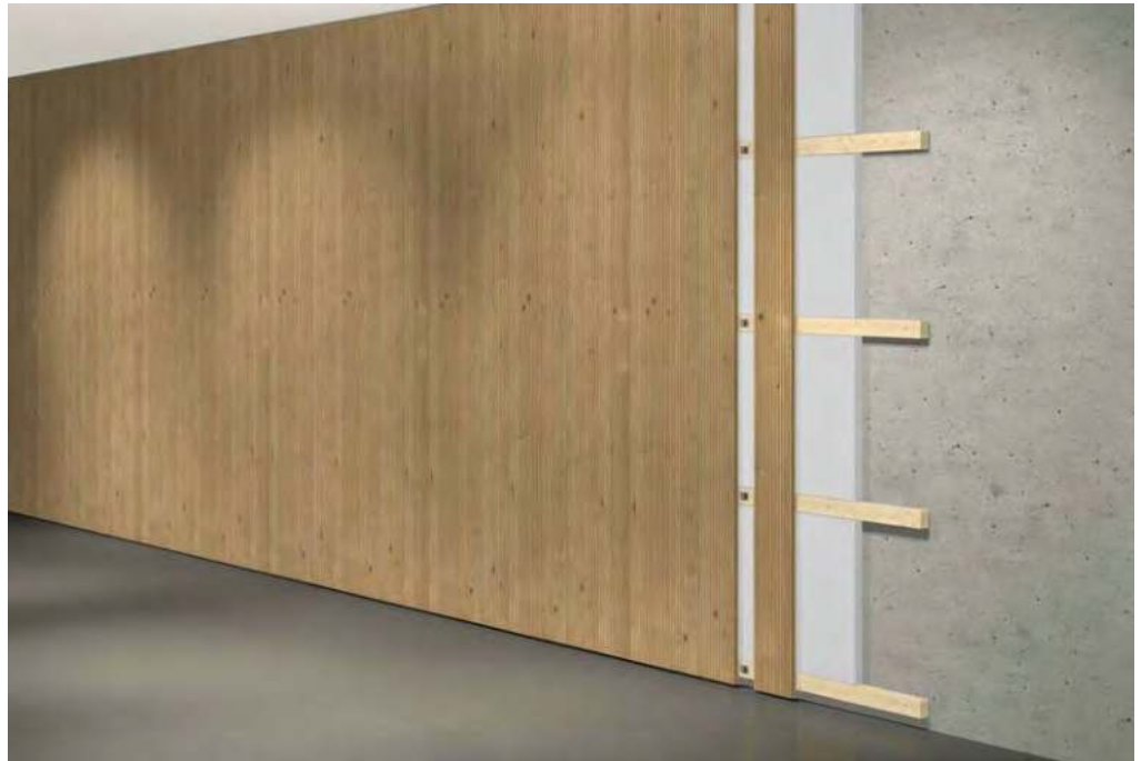
Vertical assembly without offset with all-round gap.
